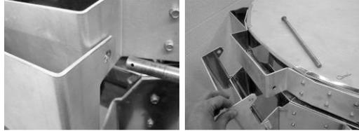
5./ Remove the eight screws on both sides of the arm support by using a 1/4" Nut Driver or Multi bit screw driver.
