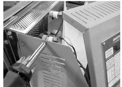
Use needle nosed pliers to pull the connectors off of the relays. Do not tug on the wires themselves.
