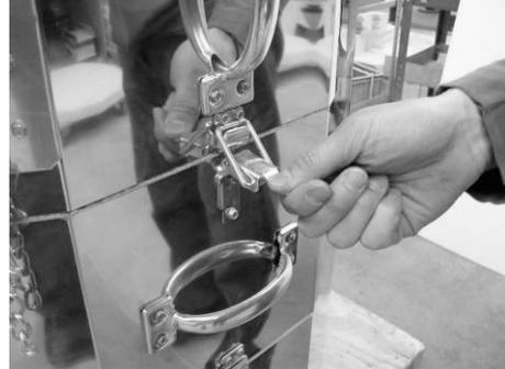
Move the kiln rings section by section.
