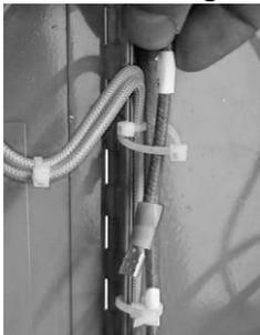
For 3 section kilns, you may also have to disconnect the 2 black wires between the middle section & Bottom section. You will need pliers and an allen key.
